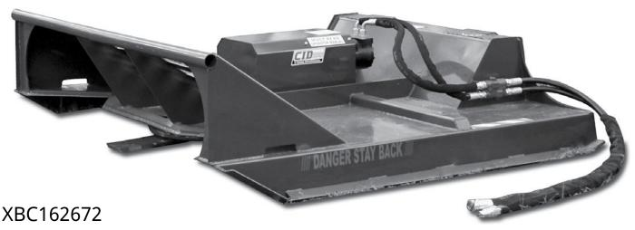
Our X-treme Brush Cutter is an ideal attachment for tough clearing applications. The cutter comes in a 60" or 72" cutting width. It is equipped with bidirectional blades, powered by a high torque motor and features a 100-hp Omni gear box. A flow of 14–20 gpm is required on the low flow, 20–30 gpm on the mid flow, and 30–50 gpm on the high flow. The one year warranty does not cover the blades or hoses. (Please see page 65 of the catalog for full warranty).
